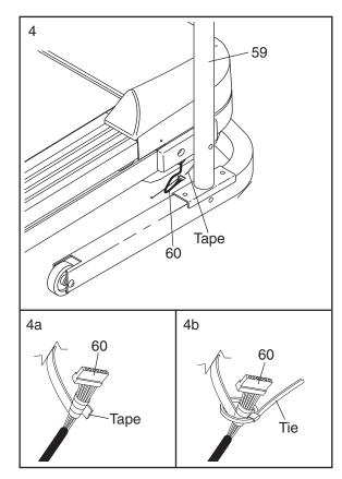
5. Carefully pull the opposite end of the tape to pull the Wire Harness (60) up through the Right Handrail (59) and out of the hole in the side of the Right Handrail.
